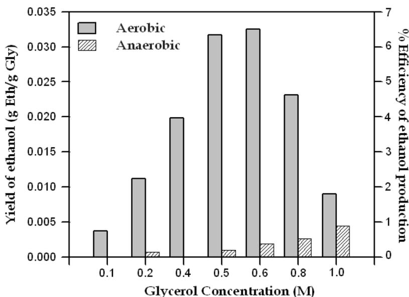
Figure 2: Effect of glycerol concentration on bioethanol production (at pH 5 & 24 hours)
