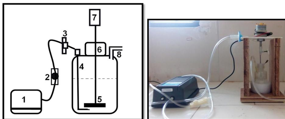
**Figure 1: Small scale bioreactor – Schematic sketch and Fabricated bioreactor (1: Air pump, 2: Air flow controller, 3: Micro filter, 4: Needle Sparger, 5: Agitator, 6: Lid / cap, 7: Motor, 8: Air vent)**
