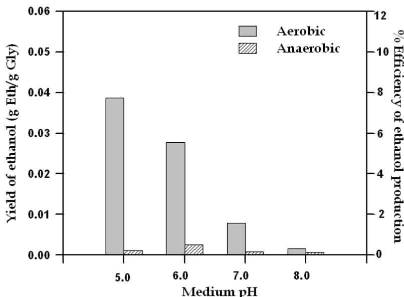
Figure 3: Effect of pH on bioethanol production (at 0.6M glycerol concentration & 24 hours)
