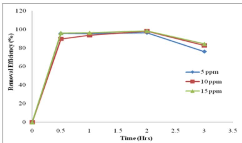
Figure.9. Variation of removal efficiency of lead with respect to time
