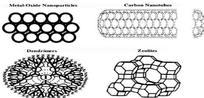
Figure 1. Selected nanomaterials currently being evaluated as functional materials for water purification (Courtesy: Savage and Diallo 2005)
