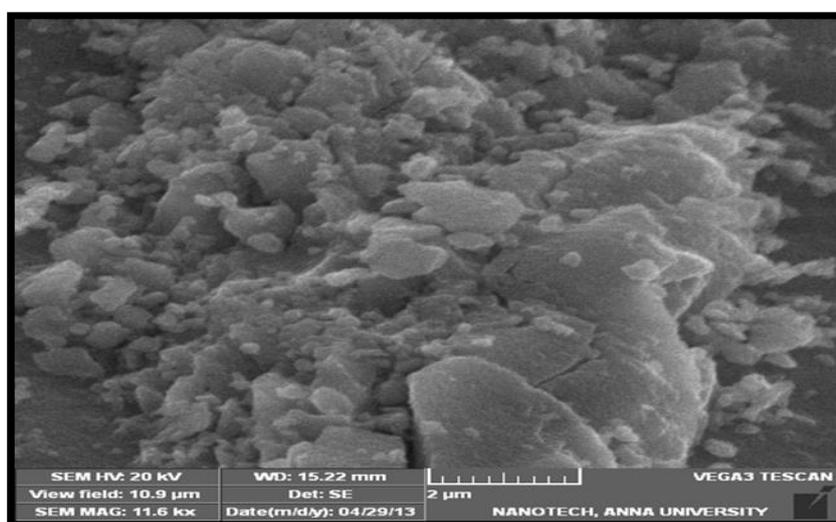
Figure.6 SEM Image of Titanium Dioxide Particles
