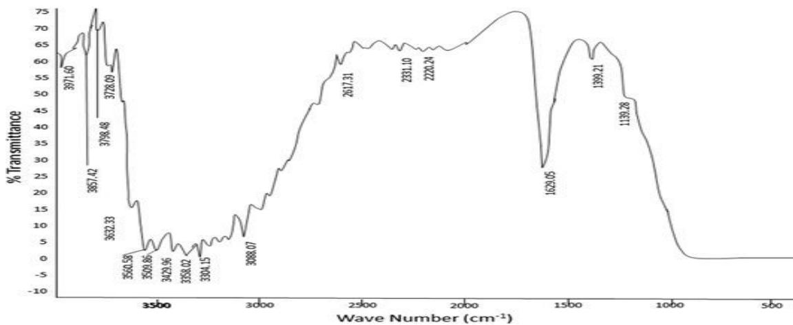
Figure 4. FTIR spectra of TiO2
