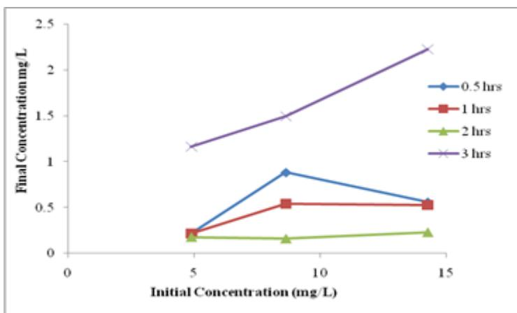
Figure.8. Variation of final concentration of lead with respect to initial concentration of lead
