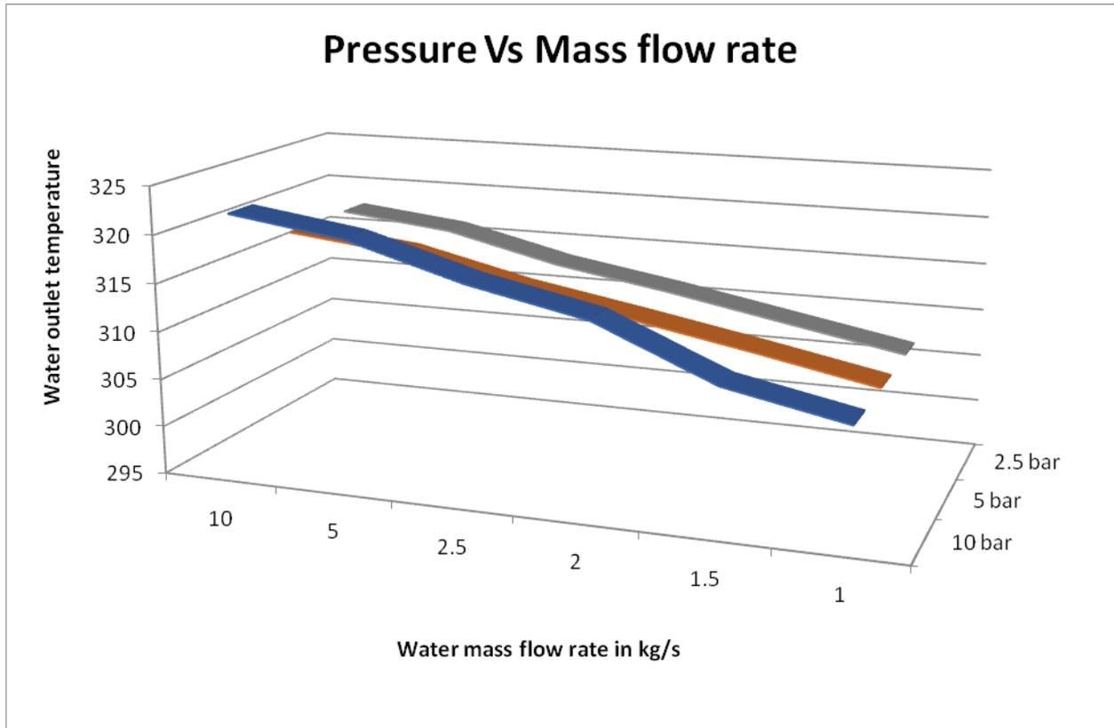
Fig 6: Graphical representation of water outlet temperature for varying pressure and mass flow rate
