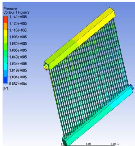
**Fig 4: Pressure contours**
