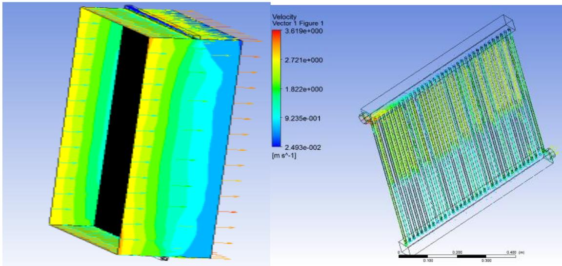
**Fig 3: Velocity vector of air and water**
