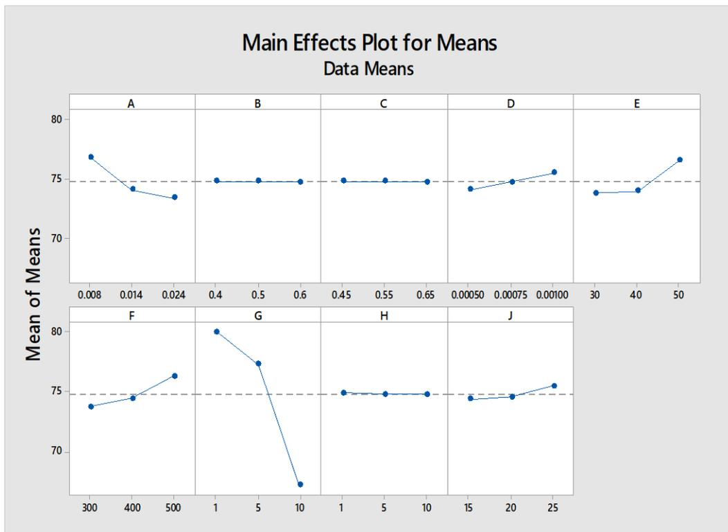
Fig 7: Mean effect of parameters to water outlet temperature
