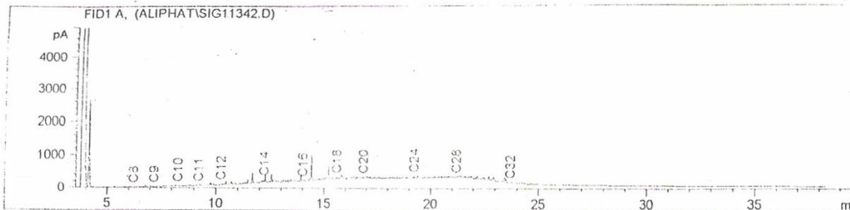
Figure 2: Chromatographic profile of TPH for *Oscillatoria sp* at day 21 (dark phase)
