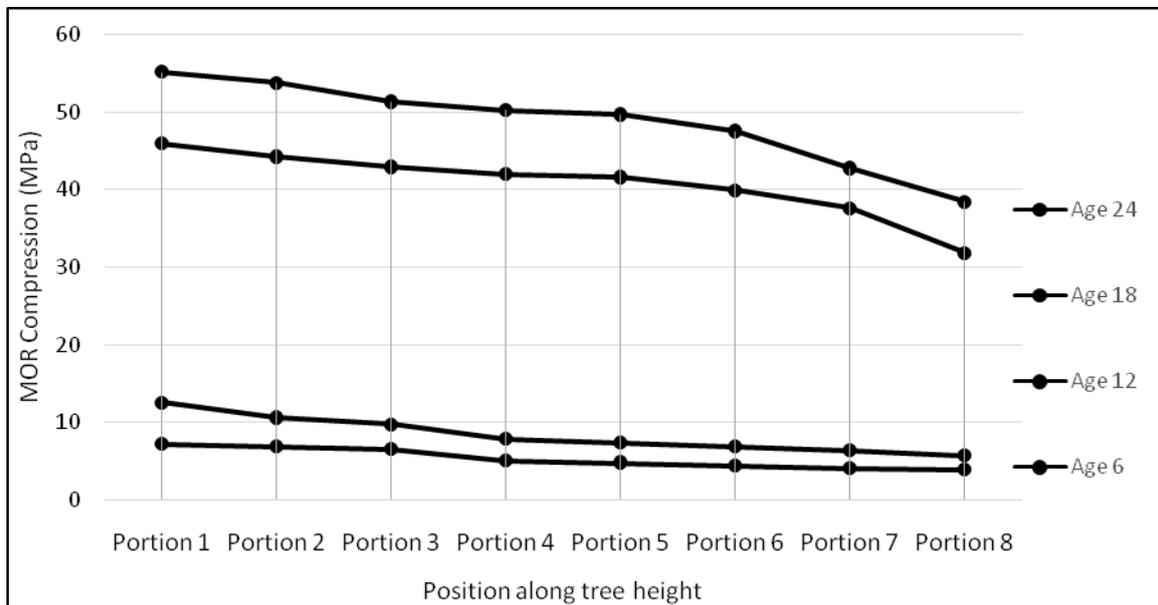
**Figure 3: The modulus of rupture on compression tests at various age-group of cultivated *C. manan* at portions height 1 to 8**
