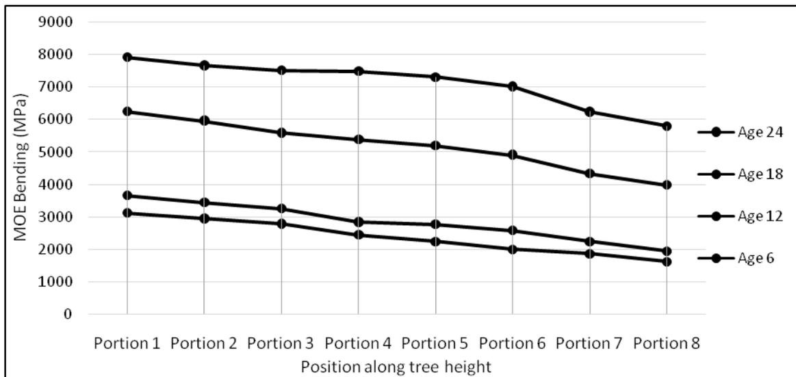
**Figure 5: MOE on static bending tests at different age-group of cultivated *C. manan* of portions height 1 to 8.**
