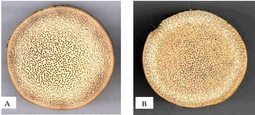
**Figure 1: The cross-section is showing a distinct variation in density between an outer and inner part of cultivated 24 years-old (picture A) and a 12 year-old *C. manan*.**
