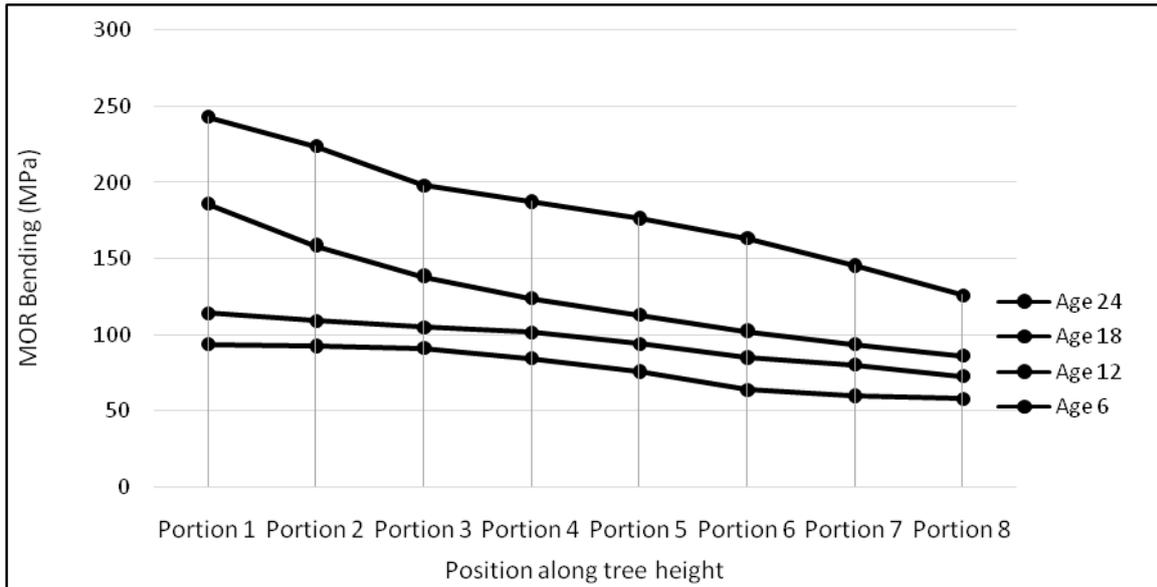
**Figure 4: The modulus of rupture on bending tests at different age-group of cultivated *C. manan* at portions height 1 to 8.**
