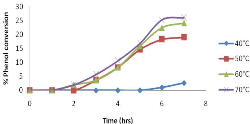
**Figure 2: Effect of temperature on the oxidation of phenol**
