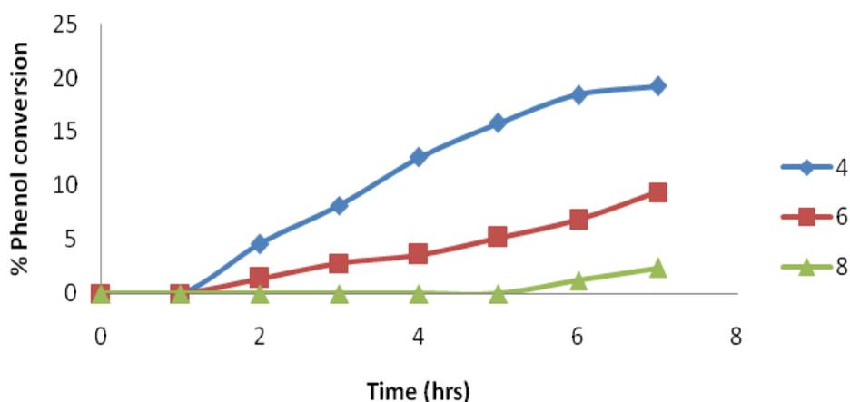
Figure 4 Effect of solvent volume on % phenol conversion
