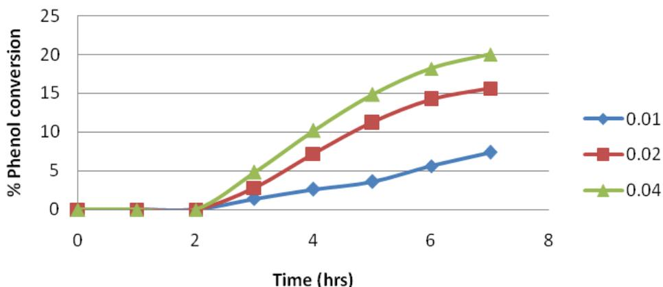
Figure 5: Effect of catalytic amount on % phenol conversion
