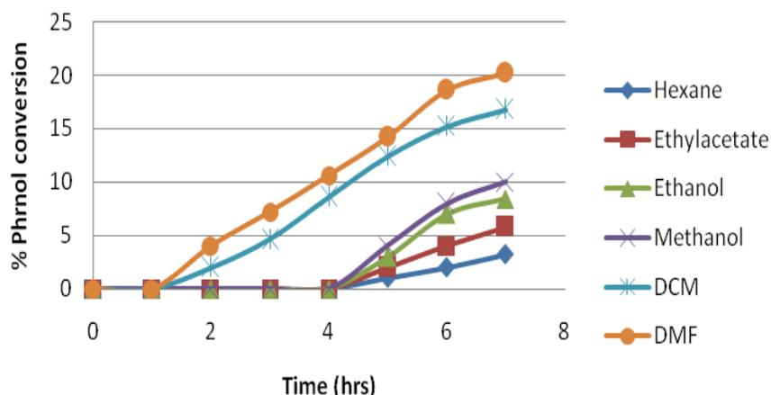
**Figure 3: Effect of different solvents on the oxidation of phenol**
