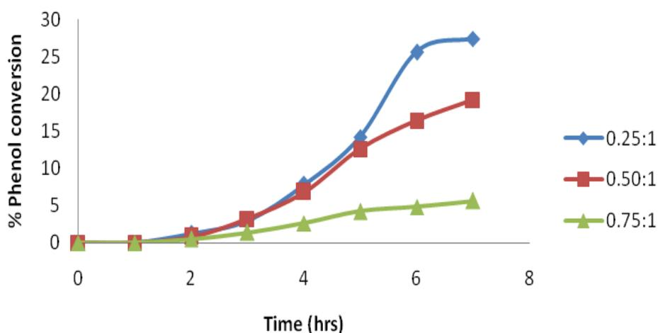
**Figure 1: Effect of hydrogen peroxide: phenol molar ratio on % phenol conversion**
