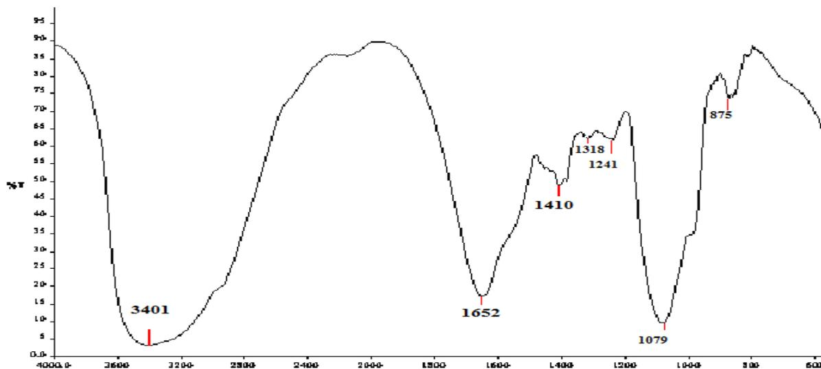
Fig. 4. FTIR spectra of biostabilized PdNPs
