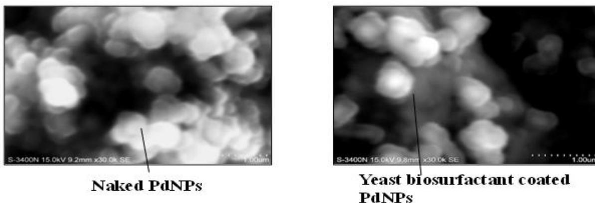
Fig. 2. Scanning electron micrograph of (a) naked PdNPs and (b) biostabilized PdNPs synthesized at 60° C.
