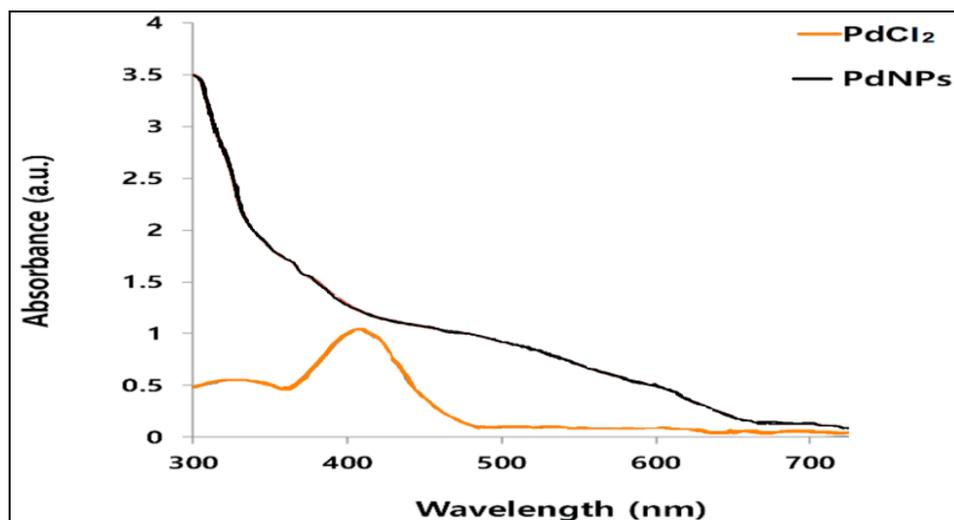
Fig. 1. UV-Vis spectra of PdCl<sub>2</sub> solution and biostabilized PdNPs
