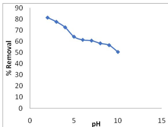
Fig 4: % colour removal at different pH
