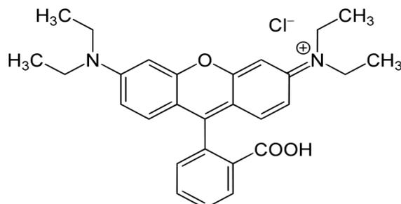
Fig 1: Rhodamine-B dye structure
