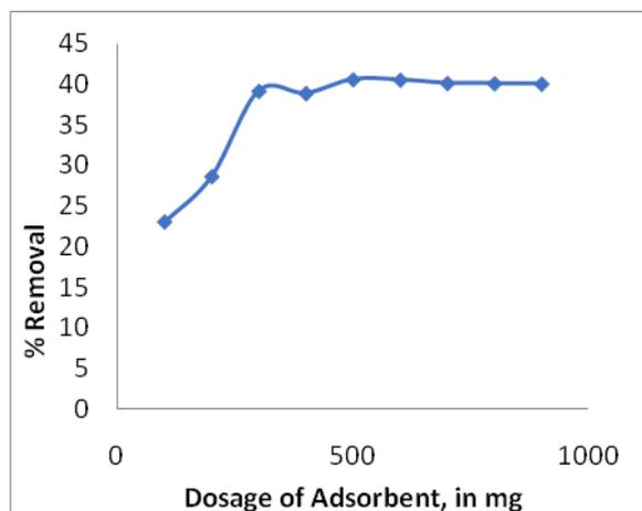
**Fig 2: Dosage of the Adsorbent v/s % Colour Removal**
