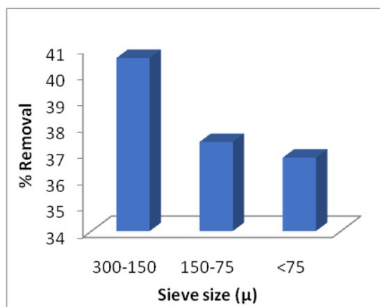
**Fig 3: % Colour Removal v/s Particle size of sawdust**
