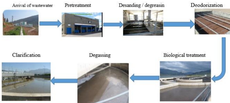
Figure 2: Wastewater treatment steps in Sidi Merouane plant
