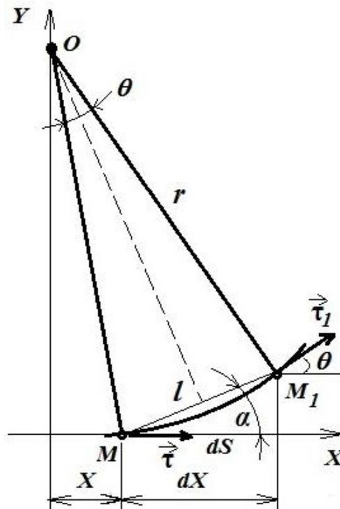
Figure 4: Scheme for analyzing the shape of the longitudinal profile of the wedge working surface
