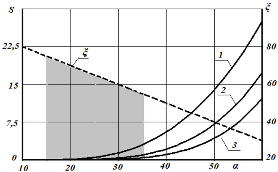
Figure 7: Dependences of the change in the profile  $S$  of the surface of the paw opener when the soil element moves along the curved surface of the wedge from the angle of the wedge  $\alpha$  for different curvature radii: 1 -  $r=10$ cm; 2 -  $r=25$ cm; 3 -  $r=40$  cm
