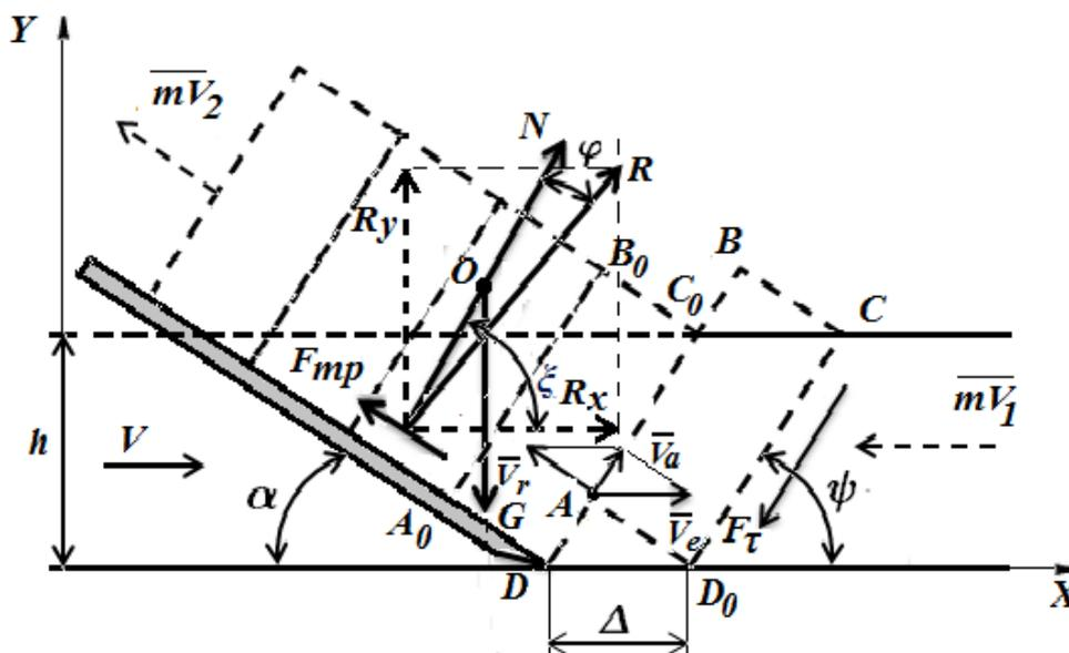
Figure 1: Calculation model of interaction flat wedge with soil
