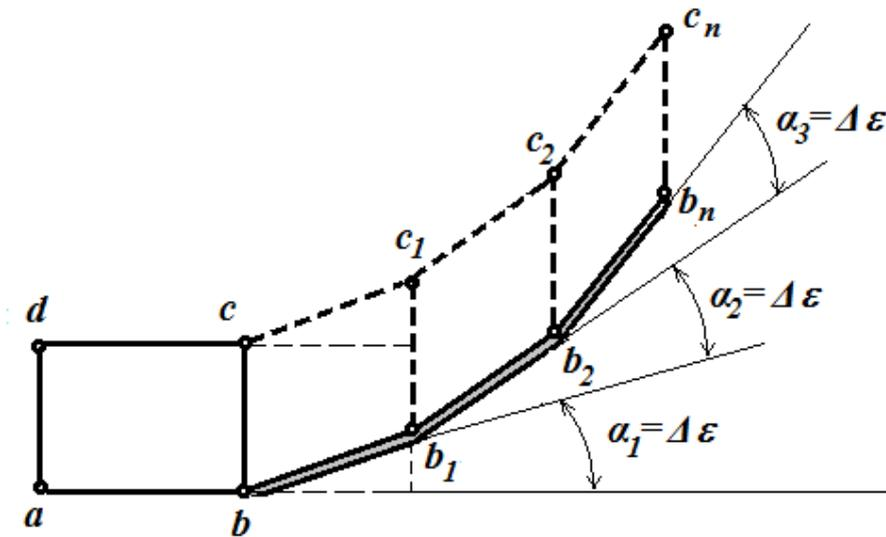
Figure 3: Scheme of deformation soil layer by a concave wedge with varying angle  $\alpha_n$
