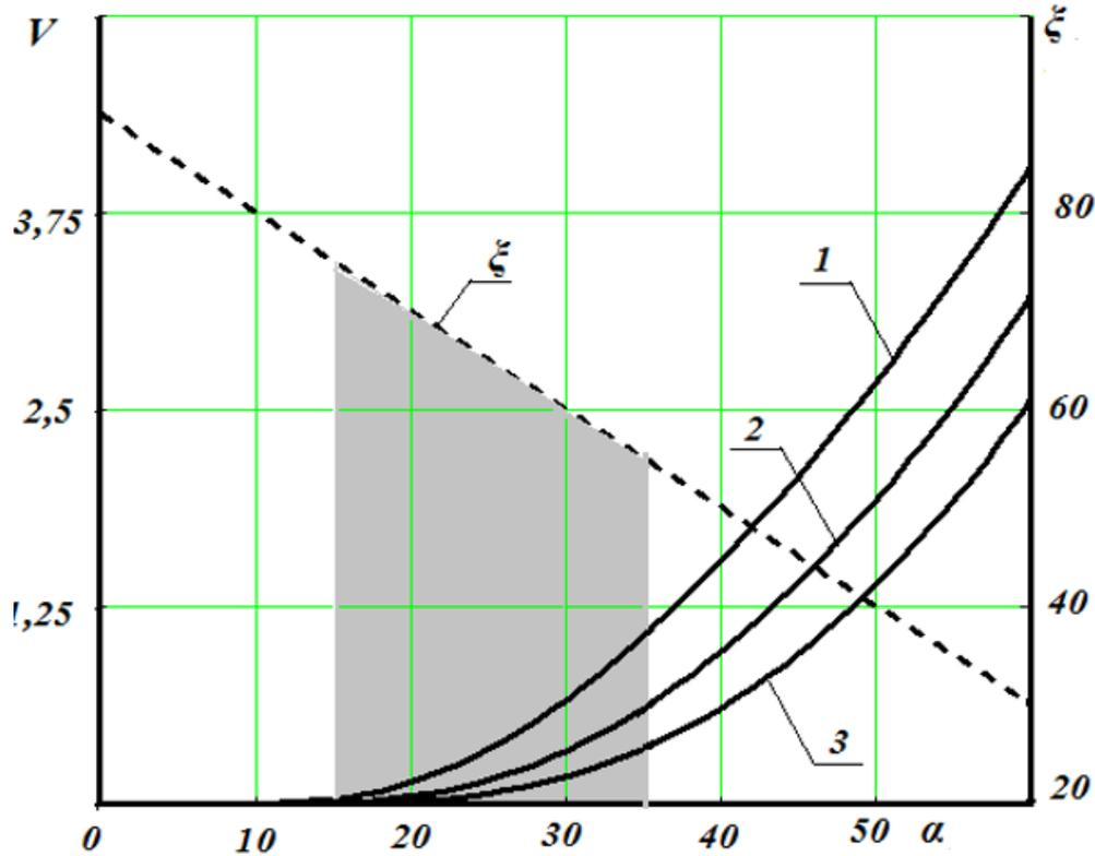
Figure 6: Dependences of the change in the speed  $V$  of the motion of the soil element along the curved surface of the wedge from the angle of the wedge  $\alpha$ , for different values of the coefficient of friction: 1-  $f=0,4$ ; 2 -  $f=0,5$ ; 3-  $f=0,6$ .
