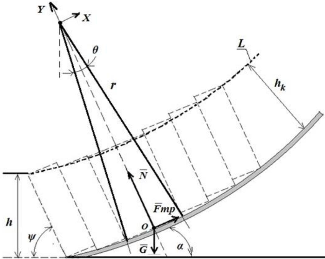
Figure 5: The calculation scheme of interaction curved wedge with soil
