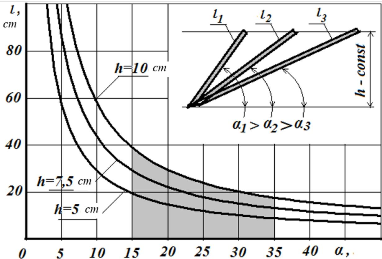
Figure 2: Dependence of the wedge length  $l$  on the angle of its setting  $\alpha$
