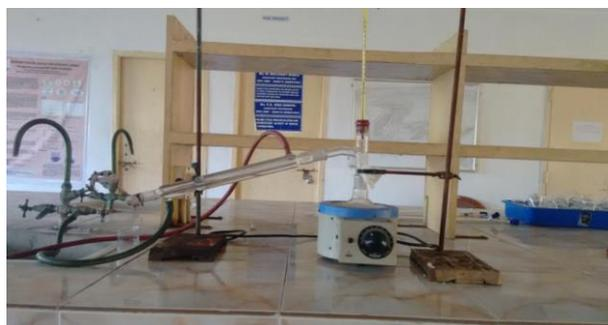
Fig 1: Solvent Extraction Apparatus
