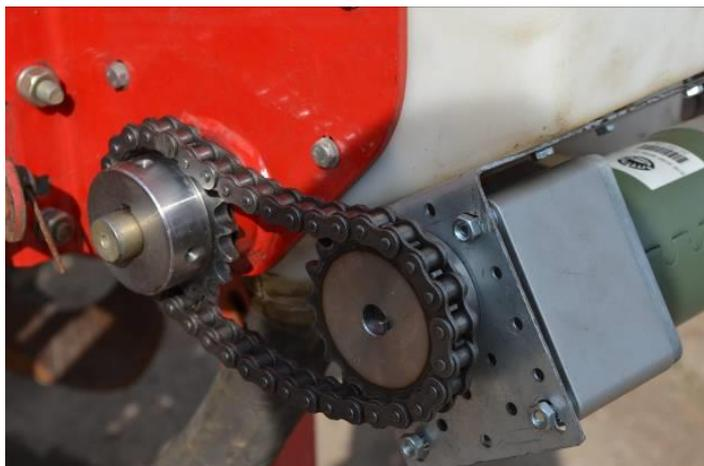
**Figure6: A dosing unit in working position**
