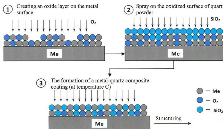
**Figure 2: The complex processes of changing the chemical and phase composition of the metal-quartz composite material**
