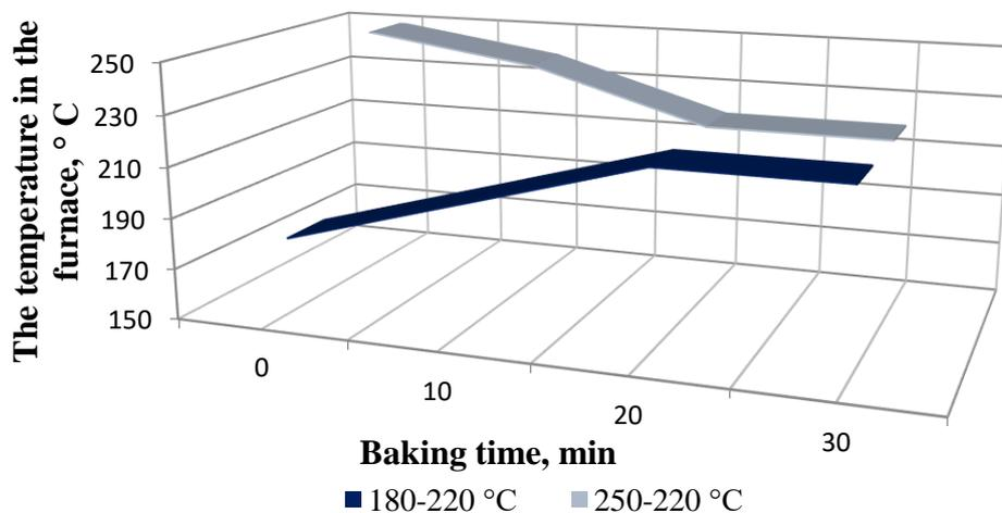
**Figure 4: Temperature variation with various baking options.**
