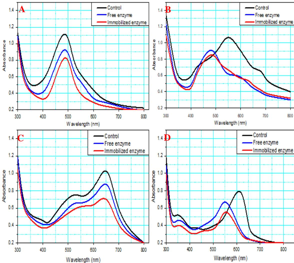
Figure (5): Synthetic dyes decolorization with immobilized laccase (IL) in presence or absence of 2 mM PG-redox mediator. (A) CR; (B) RBBR; (C) MB; (D) MG were incubated at 30 °C for 24 h.
