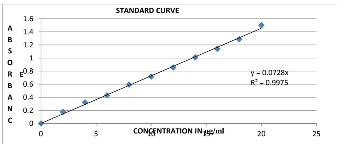
**Figure 3: Calibration Curve for Amphotericin B**
