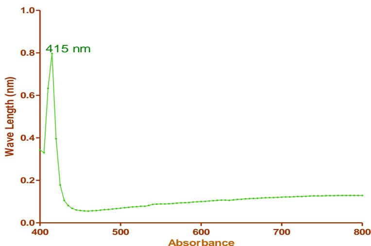
Figure 2: Determination of  $\lambda_{\text{max}}$  of Amphotericin B
