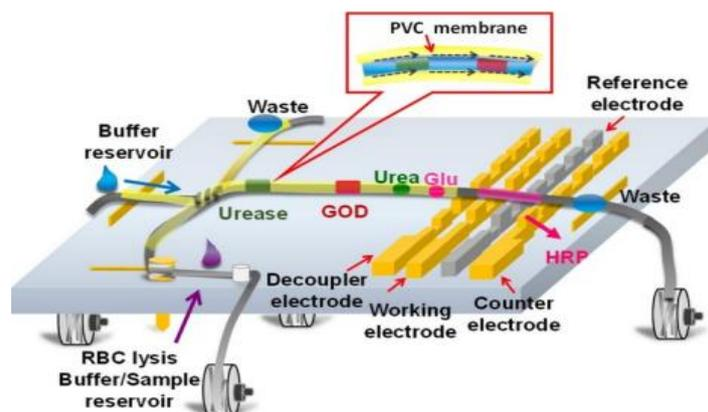
**Figure.1. Schematic of the enzyme-doped thread coated with PVC membrane for high-performance CE-EC detection.[9]**
