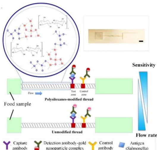
**Figure 10. Analysis of food safety via new point-of-care (POC) technologies. A thread-based colorimetric detector was developed to detect *Salmonella enterica* in food items includes lactose, lettuce and orange juice.[20]**
