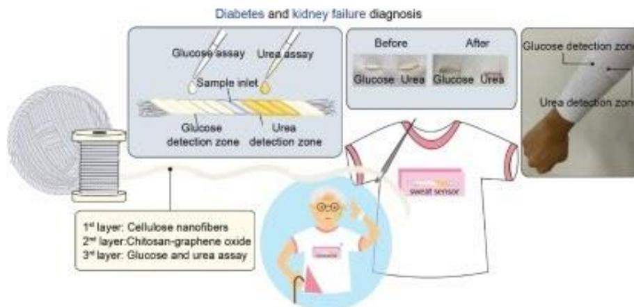
**Figure 7. Abstract procedure of the fabricated cotton thread-based biosensor. [16]**
