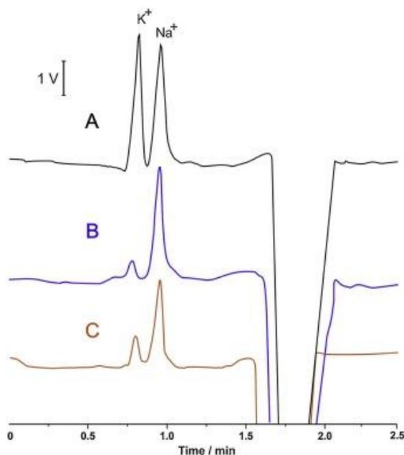
**Figure 11. Electropherograms of (A) a standardized solution of  $K^+$  and  $Na^+$  (75 mol L<sup>-1</sup>); (B) a 100-fold diluted lemon and (C) a 100-fold diluted cola diet soft drink..[24]**
