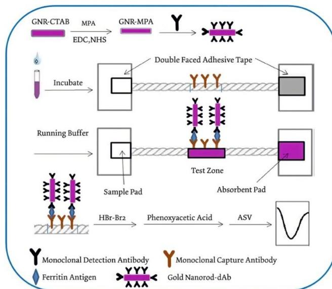
**Figure 5. The principle of the nature cotton thread-based immunoassay device for electrochemical detection of ferritin[15]**
