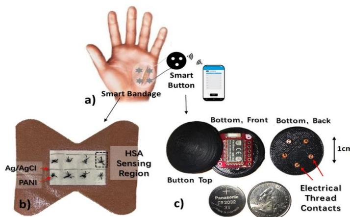
**Figure 6. System Overview. Wireless data transmission from smart bandage to phone (a). Closer view of fabricated thread-based pH sensing bandage with HSA sensing regions as working electrodes and Ag/AgCl thread as reference electrode (b). Readout electronics encased in a 3D printed button and smartphone application for data acquisition © ref[12]**
