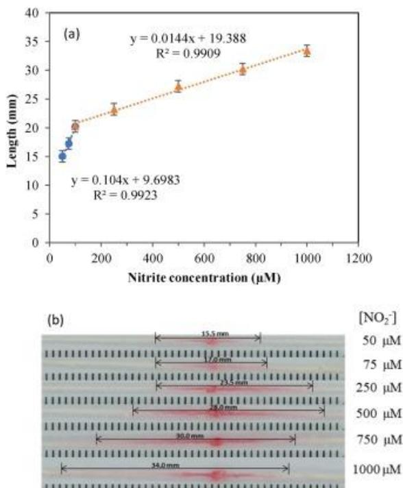
**Figure9. (a). Thread-based platform calibration curve for nitrite measurement and (b). Image of threads is used to detect nitrite at concentrations. [21]**
