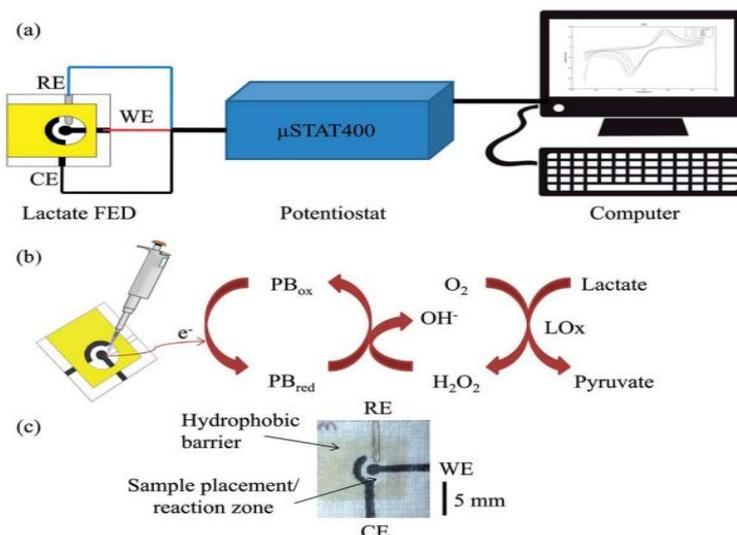
**Figure 4. Overview of FED technology. (a) The instrumental setup for lactate determination. (b) The reaction that occurs at the C-PB/LOx electrodes of the FED. (c) Picture of the fabricated FED (15-15 mm). RE, reference electrode; WE, working electrode; CE, counter electrode.[13]**
