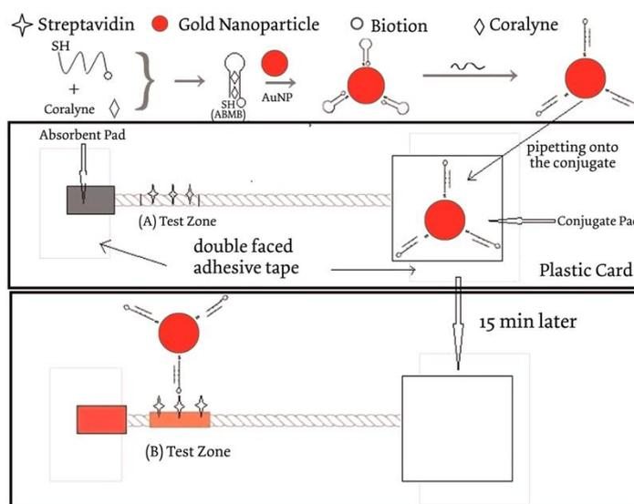
**Figure 8. The principle of the cotton thread-based device for DNA detection[17]**
