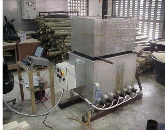
**Figure 6: An electrical oil heat treatment machine**
