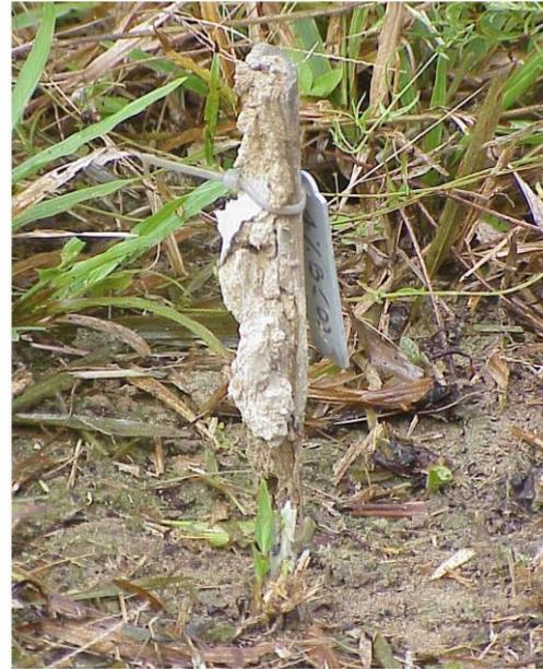
**Figure 8: Ground testing of bamboo showing severe termites attacks**
