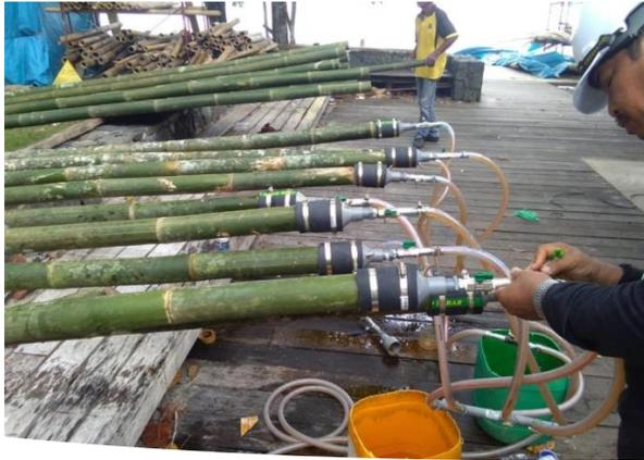
**Figure 5: Preservation of the bamboo culms through sap-displacement technique**
