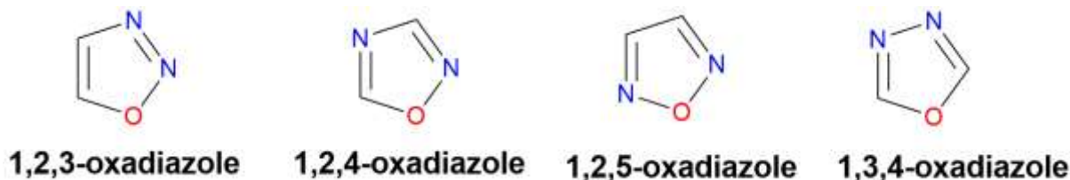
Figure 1: Chemical structure of four different isomer of oxadiazole
